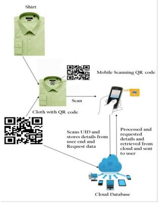
Figure 2. Basic working of the system [8]
